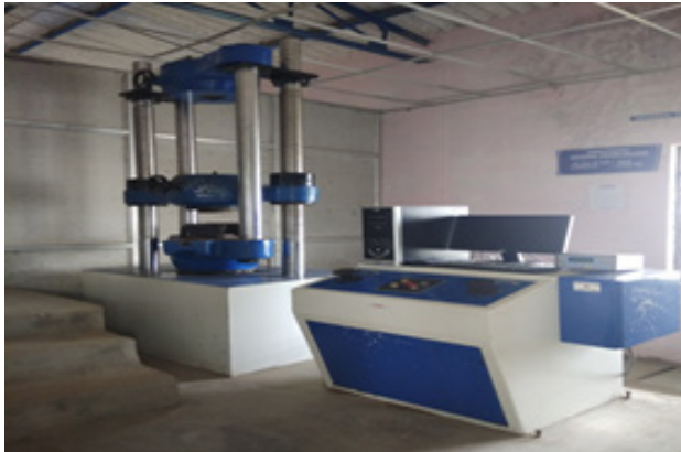
Computerised Universal Testing Machine (UTM) -100 Tonnes capacity
